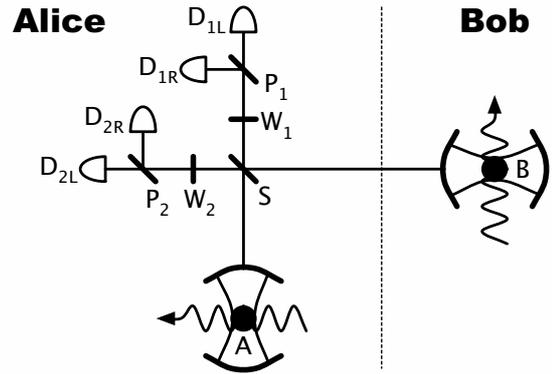
Figure 1: Experimental scheme to teleport the internal state of atom *A* to atom *B*. *S* is a beamsplitter, *W*<sub>1</sub> and *W*<sub>2</sub> are quarter wave plates, *P*<sub>1</sub> and *P*<sub>2</sub> are polarization beam splitters, and *D*<sub>1L</sub>, *D*<sub>2L</sub>, *D*<sub>1R</sub>, and *D*<sub>2R</sub> are photodetectors. Each winding arrow represents the classical driving field
